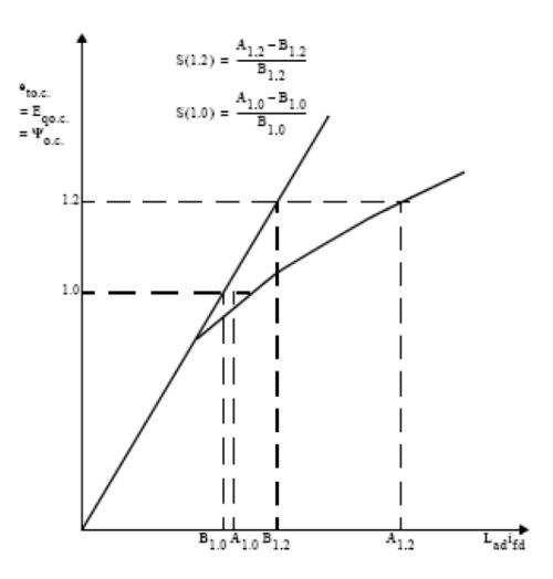
Magnetic saturation data to be assumed S(1.0) =S(1.2) = Acceptable IEEE standard excitation model available with PSS/E simulation package
